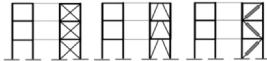
Figure 11.5 – Frames with buckling restrained bracings (dissipative zones in tension and compression diagonals)
