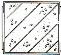
confinement through FRP or steel collars
