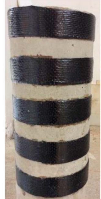
confinement through FRP jacket or strips
