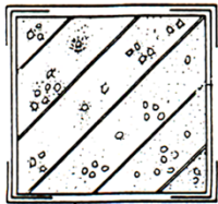
confinement through FRP or steel collars
