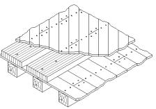
(f) Timber planks and additional floorboard overlay
