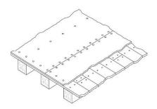
(a) Additional sheathing (diagonal floorboards) (b) Structural woodbased panel overlay
