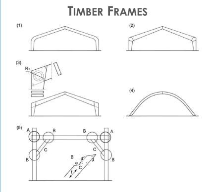
**Figure 10.3**— Timber frames addressed: 1) frames with relatively thin lamellas (glued), 2) finger joint (glued) connections, 3) dowelled connections, 4) arches, 5) traditional frames
