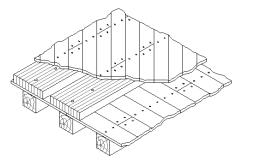
(f) Timber planks and additional floorboard overlay
