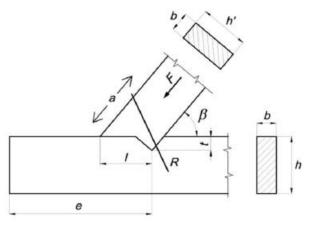
Figure C.1 — Example of reinforcement to be applied to the single-step connection
