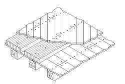
(f) Timber planks and additional floorboard overlay
