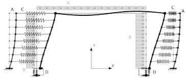
(2) If the integral abutment bridge is above-ground and in contact with approach embankments, the free-field displacements  $\delta_{\rm ff}$  should be taken equal to as given in Formula (D.5).
