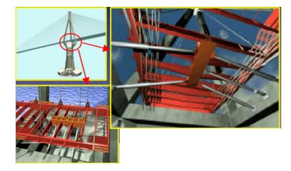
(1) In cable-stayed bridges, the deck should be continuous.
