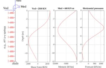
Piles that satisfy the geotechnical verifications (bearing capacity & settlements under vertical loads) may turn out to be too heavily reinforced
