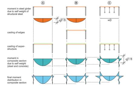
Figure 6-5: Influence of casting sequence / time of restraint
