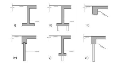
Figure 10.1 — Types of integral abutment bridges: i) full height integral abutment on pad footing; ii) full height integral abutment on piles; iii) bank pad; iv) embedded wall integral abutment; v) full height integral abutment on single row of piles; vi) bank pad on single row of piles. Other types are possible
